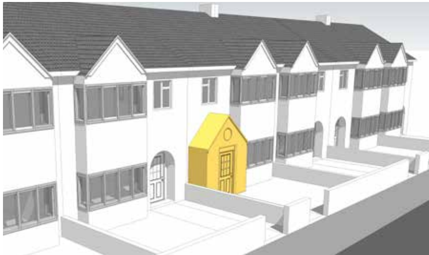
Diagram 6: Scale and design of porch is out of character within the streetscape
